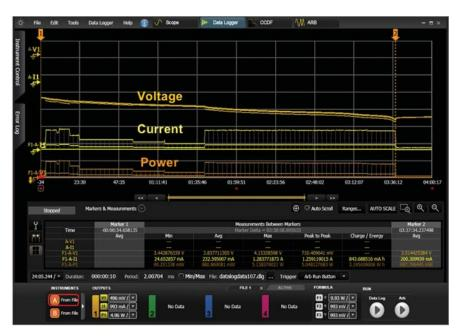
Figure 6: Data logging acquisition showing voltage, current, and power (actual battery rundown)
