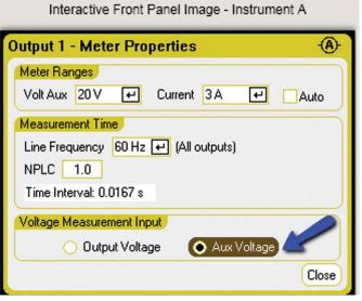
Figure 4: Auxiliary voltmeter setup
