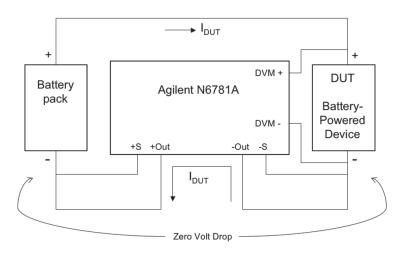
Figure 1: The recommended setup for measuring battery run-down performance using the N6781A SMU. Note that remote voltage sensing eliminates the voltage drop in the wiring between the battery pack (-) and DUT (-). In this setup, the N6781A SMU module will be installed inside an N6705B DC power analyzer mainframe.
