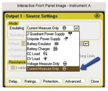
Figure 3: Source setting menu on the 14585A control and analysis software
